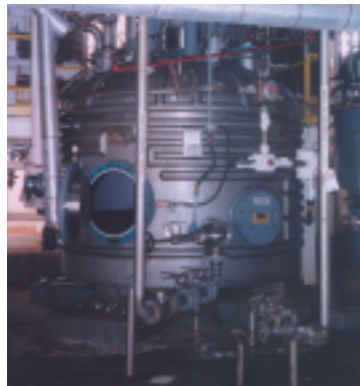
7 sq.m. 316 SS "COMBER" Filter Dryer In Plant 2
