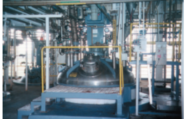
2000 Gallon 316 SS Reactor In Plant 1
