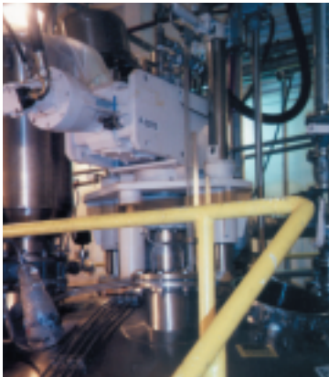
1 Of 3 Mirror Polished 7 sq.m. 316 SS "COMBER" Filter Dryer—1997
